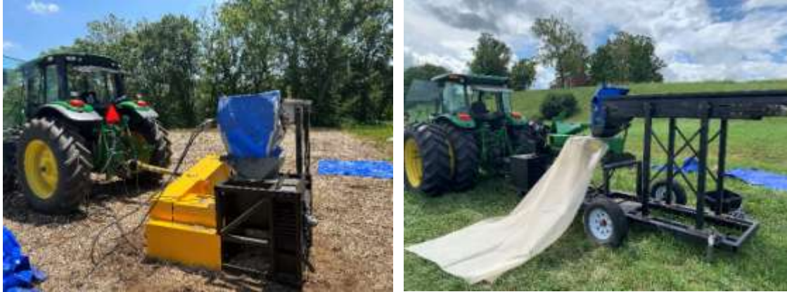
Figure 1. Setup for the integrated Harrington Seed Destructor (iHSD) (left) and Redekop Seed Control Unit (SCU) (right) test stands. Chaff was loaded on the conveyor belt and fed into the mill that was powered by the tractor power take-off (PTO). The process chaff and weed seeds were captured by the mesh bag (example right) as it exited the mill.
