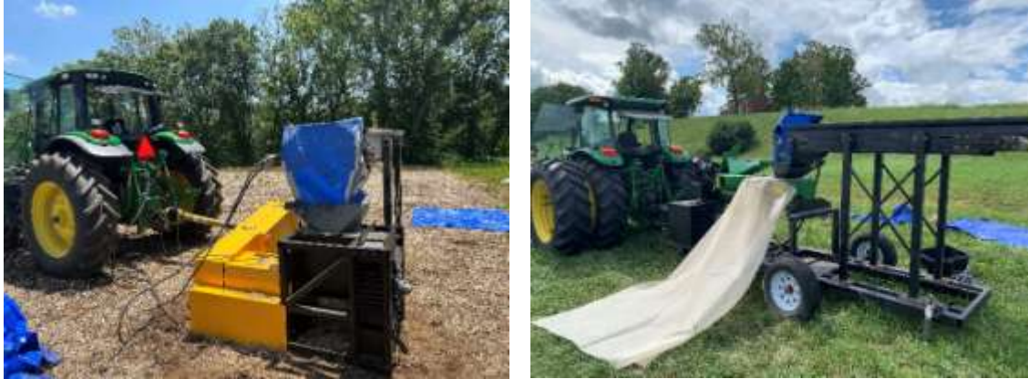
Figure 1. Setup for the integrated Harrington Seed Destructor (iHSD) (left) and Redekop Seed Control Unit (SCU) (right) test stands. Chaff was loaded on the conveyor belt and fed into the mill that was powered by the tractor PTO.
