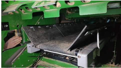
Figure 4 - Compact electric conveyor installed on the top sieve of a John Deere combine harvester.
