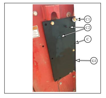
1.8 Install adaptor assembly bracket (A) to radiator/ adaptor plate (C) studs (C2), with:
