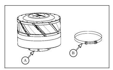
**2.1** Install KAS Pre-cleaner assembly (A) on to intake tube (F), with:
