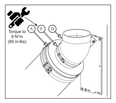
**1.10** Install air intake tube (**B**) to elbow (**D**), with: - hose clamp (**E**)
