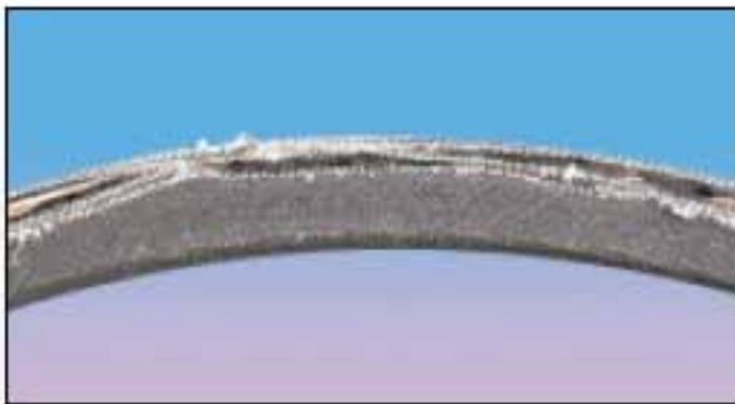
Rapid Sidewall Wear
