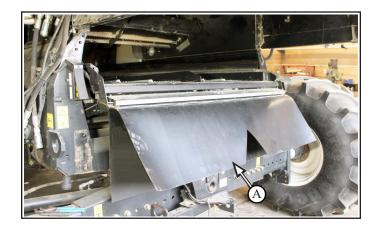
**1.2.2** Remove sieve extension assembly (**A**) from the bottom of grain loss monitor (**D**) removing existing hardware (**D1**) both sides
