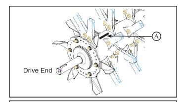
2. Straw chopper serial number plate (B):- located on the chopper wall, non-drive side, below the rotor shaft shield
