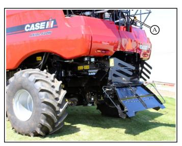
**1.9 REAR WINDROW ROLLER** (A) speed adjustment In most cases, the factory speed setting is acceptable. If required, adjust speed of rear windrow roller to suit straw discharging from the combine
