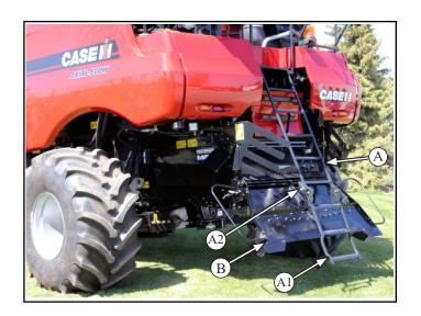
**1.8.3** Always store ladder (**A**) in the upward position when operating the straw chopper
