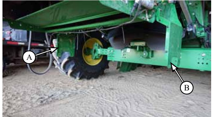
View of combine with SCU removed and side plates mounted
