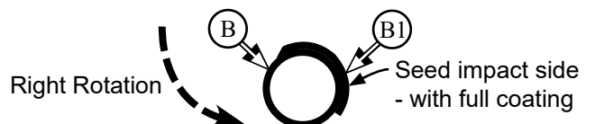
Worn out rotor from left side moved to be used as the right rotor
